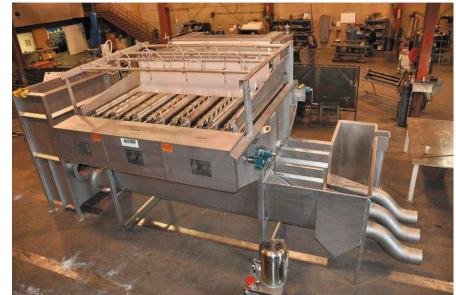
Special to the Statesman Journal Layton Potato Sizing system used for making French Fry's.
